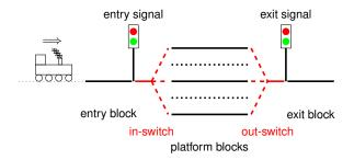
ENV0 There are platforms in between an entry block and an exit block.
