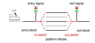
ENV3 There are switches connecting the entry/exit block to a platform.
