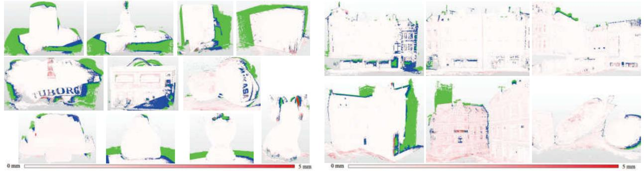
Fig. 8. Qualitative error results correspond to Fig. 7. The variation from white to red in increasing order illustrates the magnitude of the error. The points marked blue/green are masked out in the evaluation, for lacking corresponding scan data as ground-truth.
