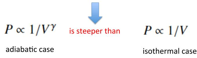
as you compress a gas adiabatically its temperature rises which increases the pressure compared to the isothermal case
