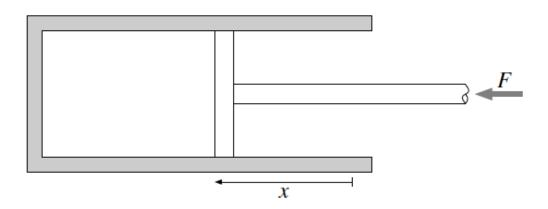
Let's consider the work done when compressing a gas with a piston. The piston is flat, has area A, and moves perpendicular to its surface. If the gas pressure is P, then the force needed to move the (frictionless) piston is F = PA.
