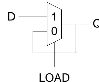
A simple transparent latch can be build around a transmission gate multiplexor
