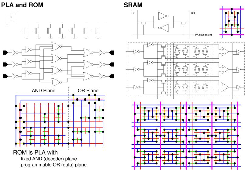
Cells are designed to butt together in two dimensions leading to efficient layout
