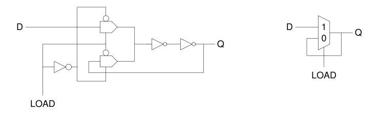
A simple transparent latch can be build around a transmission gate multiplexor
