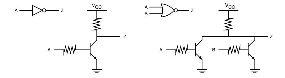
All functions can be realized using only the NOR gates<sup>1</sup> available in the RTL logic family.<sup>2</sup>
