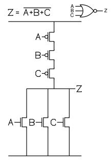
• For any set of inputs there will exist either a path to Vdd or a path to Gnd.
