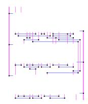
In the routing channels between the cells we route metal1 horizontally and metal2 vertically.
