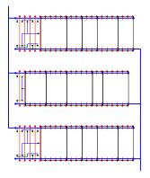
Inter-digitated power and ground rails can be routed using only one metal layer.<sup>1</sup>
