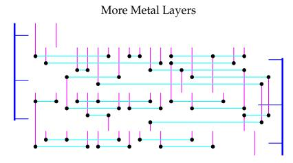
With this approach we can route safely over the cell to the specified pins leading to much smaller gaps between cell rows.
