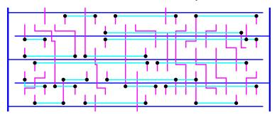
By flipping every second row it may be possible to eliminate gaps between rows. N-wells are merged and power or ground rails are shared.
