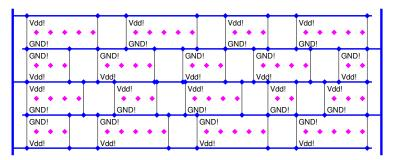
By flipping every second row it may be possible to eliminate gaps between rows. N-wells are merged and power or ground rails are shared.
