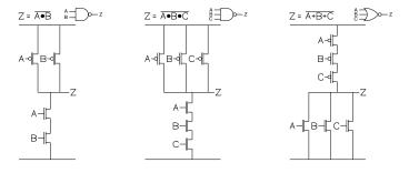
• For any set of inputs there will exist either a path to Vdd or a path to Gnd.
