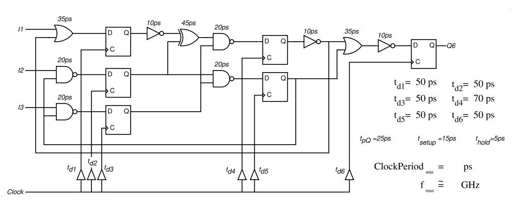
$$ClockPeriod > t_{pQ} + t_{comb-crit} + t_{setup} + (t_{d_{launch}} - t_{d_{capture}})$$
