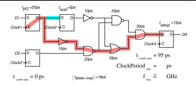
• What is the maximum operating frequency of the circuit if the clock skew is no more than 16ps?
