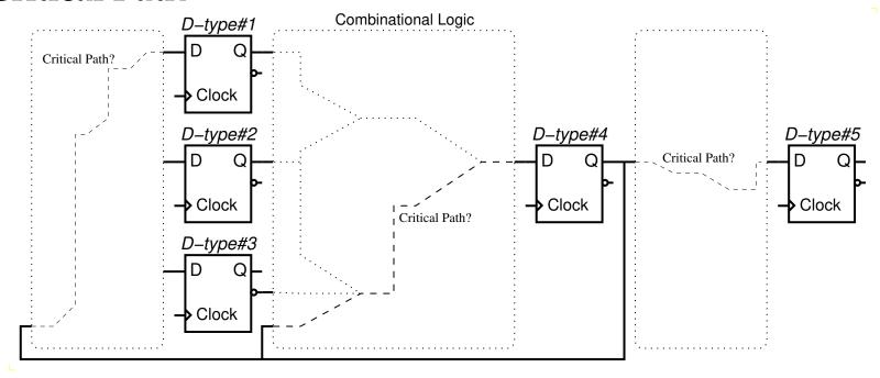
$$ClockPeriod > t_{pQ} + t_{critical\_path} + t_{setup} + (t_{d_{launch}} - t_{d_{capture}})$$
