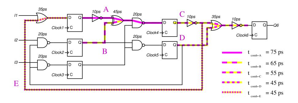
$\Rightarrow$  Initially try increasing  $t_{d4}$  by 20ps
