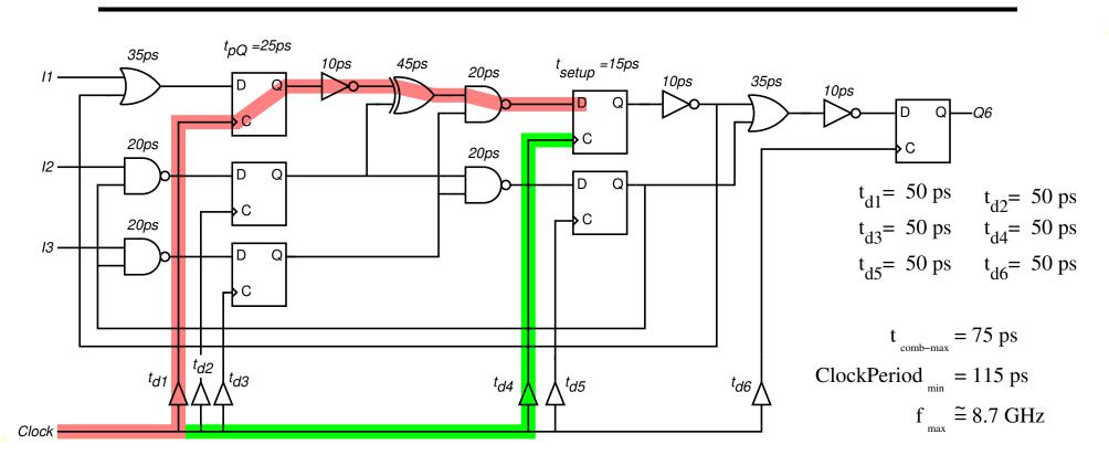
$$ClockPeriod > t_{pQ} + t_{comb-max} + t_{setup} + (t_{d1} - t_{d4})$$
