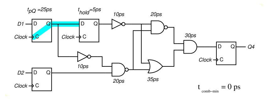
$$t_{pQ} + t_{comb-min} > t_{hold}$$
