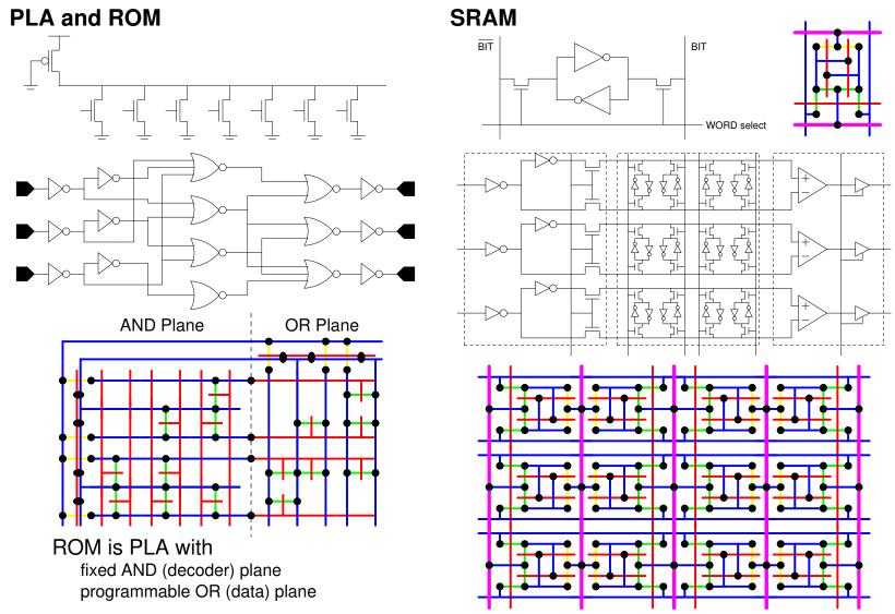
Cells are designed to butt together in two dimensions leading to efficient layout PLA layout efficiency will depend on the actual function implemented (e.g. number of common product terms)
