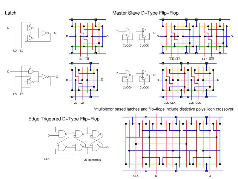
Euler path analysis is applied creatively to these multi-gate cells – gates are often linked via the common gnd/pwr node Final layouts will be more complex where clock buffers, reset circuitry and metal 2 i/o are included
