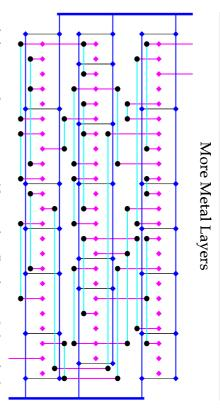
With this approach we can route safely over the cell to the specified pins leading to much smaller gaps between cell rows.
