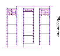
Cells are placed in one or several equal length lines with inter-digitated power and ground rails.
