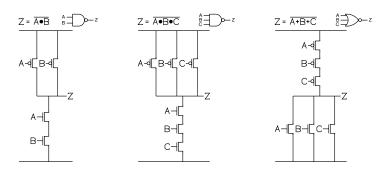
• For any set of inputs there will exist either a path to Vdd or a path to Gnd.
