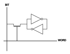
Discuss the problems associated with using this 5 transistor cell when compared to the 6 transistor version. You should consider the resolution of conflicts during operation, the sizing of transistors, and the design of associated read and write circuitry.
