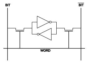
Draw a diagram showing the read and write circuitry required to support this RAM cell and briefly explain the operation of the cell for both read and write operations. Be sure to mention any conflict that may occur during read and write and explain how the sizes of the different transistors affect the resolution of such conflict.
