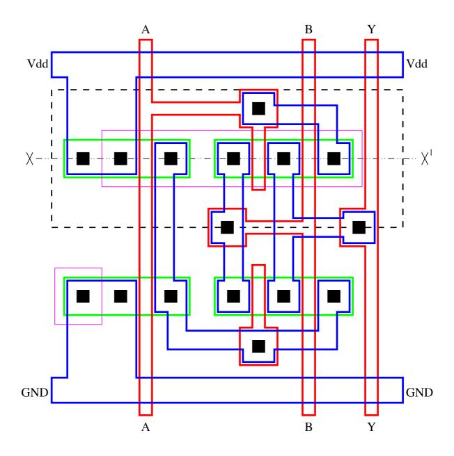
Figure B1: Mask level layout of a two-input CMOS gate
