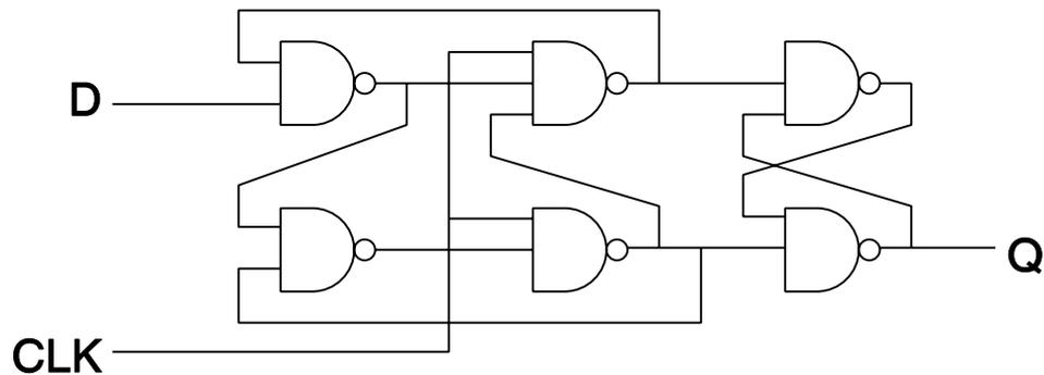
By drawing sub-circuit schematics (or otherwise), calculate the number of transistors in the above edge triggered D-type flip flop.
