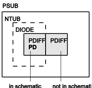
**Note:** PD is only intended for simulation of reverse leakage currents and junction capacitances. It is not recommended to use this diode as an active circuit element.
