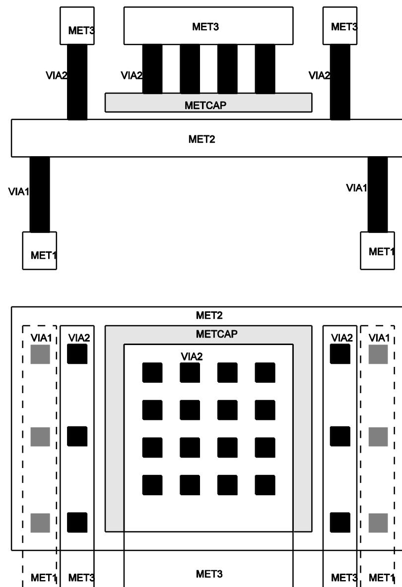
**Note:** Active and passive circuit elements under METCAP are not recommended to avoid noise coupling or deviated MIM capacitance.
