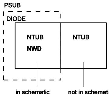
**Note:** NWD is only intended for simulation of reverse leakage currents and junction capacitances. It is not recommended to use this diode as an active circuit element.
