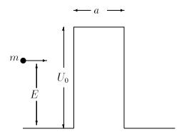
Inside the barrier, where the potential energy is  $U_0$ , the kinetic energy is  $E - U_0$  and so that the momentum, which is given by
