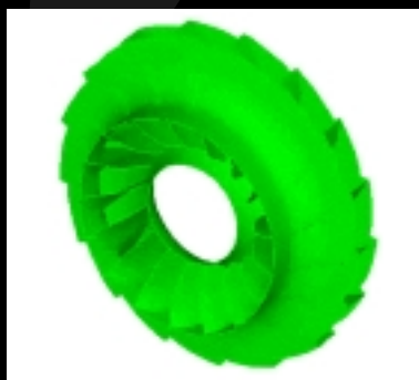
A continuously shrouded blade assembly with cyclic symmetry.
