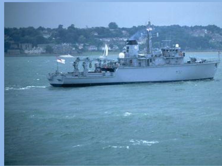
Figure 1: Mine countermeasure vessels using glass-balsa sandwiched structures
