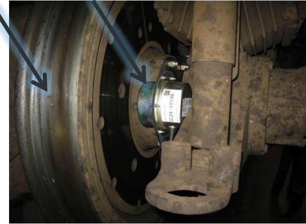
Showing sensor node bolted to train (OB right)
