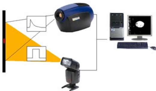
Figure 1 Experimental set up for PPT showing square wave pulse application and thermal decay data collection.
