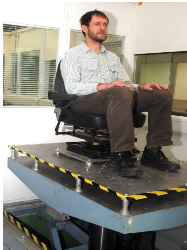
Investigating vibration effects using the vertical vibrator
