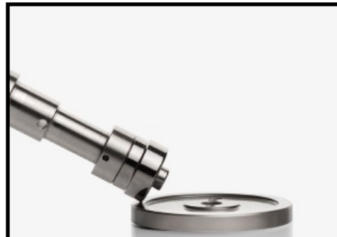
BARREL SPECIMEN FITTED ON MTM SHAFT
