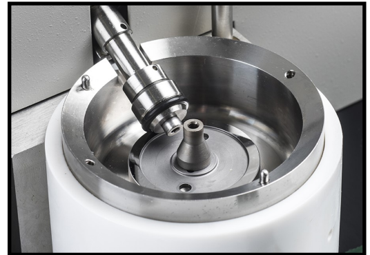
O RING HOLDER IN PLACE IN MTM2 FOR O RINGS OF SECTION 3 MM, ID 12.5 MM
