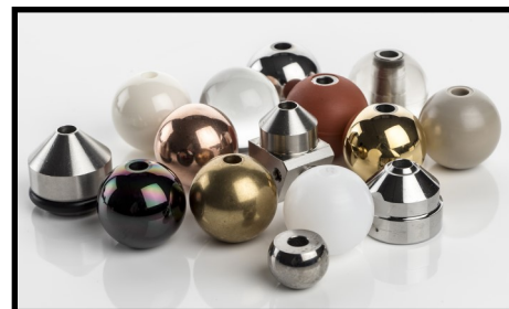
VARIOUS UPPER SPECIMEN OPTIONS FOR THE MTM
