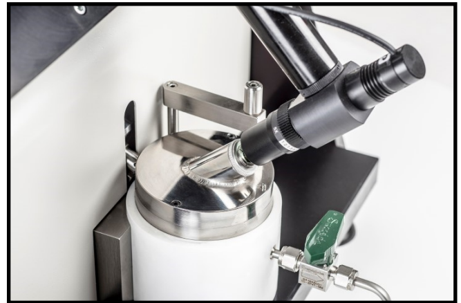
3D-SLIM MOUNTED ON THE MTM2
