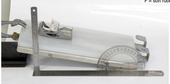
The **coefficient of friction** (static or kinetic) is a measure of how difficult it is to slide a material of one kind over another; the coefficient of friction applies to a pair of materials, and not simply to one object by itself.
