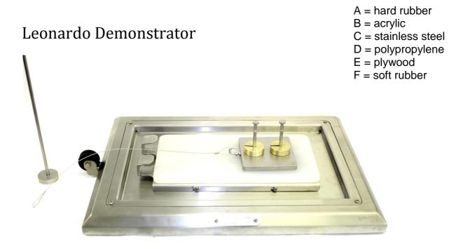
The **coefficient of friction** (static or kinetic) is a measure of how difficult it is to slide a material of one kind over another; the coefficient of friction applies to a pair of materials, and not simply to one object by itself.
